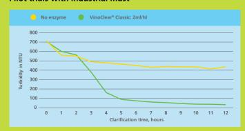
The must treated with VinoClear Classic clarifies fast, reaching a turbidity of < 100 NTU within less than five hours. Efficient depectinization is important to achieve a quick clarification, either static or forced (centrifugation, flotation). Fermenting clear must makes it possible to maintain a fresh and fruity aroma.
