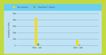
After 24 hours, the must treated with VinoClear Classic is very low in turbidity. Sediment volume is 4% (8% after 12 hours).
