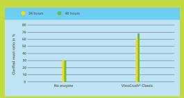
The clarified must yield is significantly increased by applying VinoCrush Classic. The speed of clarification can be improved by adding 2 ml/hl VinoClear Classic after the press in the clarification tank to help reduce the volume of lees.
